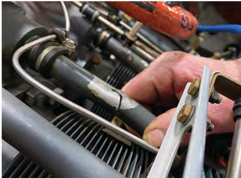
A STUCK EXHAUST VALVE caused a bent pushrod and broken pushrod housing on this Lycoming engine.
