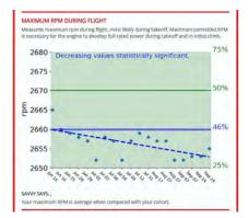
The report showed a statistically significant downtrend in takeoff rpm for Jack's airplane. Jack's Continental IO-550-N engine requires 2,700 rpm to achieve its maximum rated takeoff power of 310 horsepower. We start getting concerned if the airplane can't make at least 2,680 rpm. Jack's trend report showed that his takeoff rpm was around 2,660 in mid-June and drifted down to nearly 2,650 by mid-September—considerably out of tolerance and representing a loss of five to 10 horsepower.
