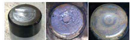
Failed Lycoming rotator cap (left) resulted in a hot spot on this exhaust valve (center). Lapping the valve in place and installing a new rotator cap resulted in a healthy looking valve 10.7 hours later.
