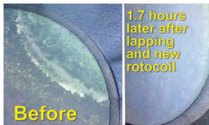
Badly burned exhaust valve, and the same valve 1.7 hours after the valve was lapped in place and the failed rotocoil replaced.
