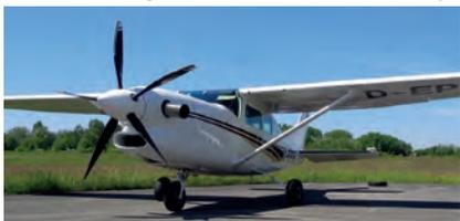
Cessna 206 Series with PT6A and 5-blade Propeller MTV-5
