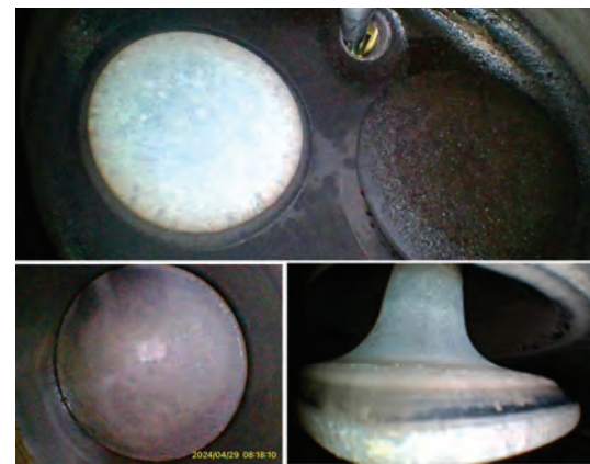
Borecope images of the number 2 exhaust valve appeared perfectly normal.
