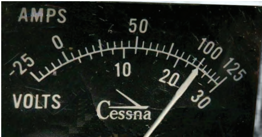
Understanding how the Cessna 310 volt-amp indicator works and what it indicates are key to diagnosing any potential problems.
