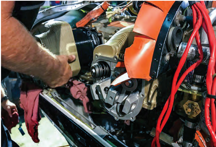
Replacing a cylinder might take a mechanic-trainee four hours to accomplish, but it certainly shouldn't require four hours of hands-on supervision by an A&P, especially if the trainee has done it a dozen times before.
