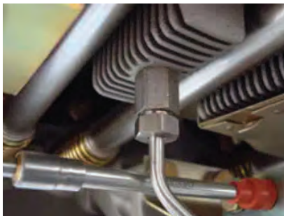
Analysis of the engine data showed that the number 6 CHT sensor or its associated connector had failed.
