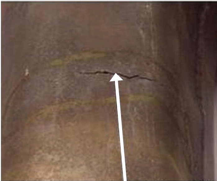
These exhaust cracks are the sort of thing we were worried about when we advised the Cirrus owner to have a Cirrus-knowledgeable mechanic inspect the engine compartment before further flight.
