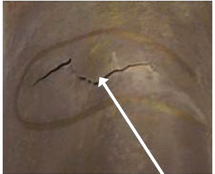
These exhaust cracks are the sort of thing we were worried about when we advised the Cirrus owner to have a Cirrus-knowledgeable mechanic inspect the engine compartment before further flight.
