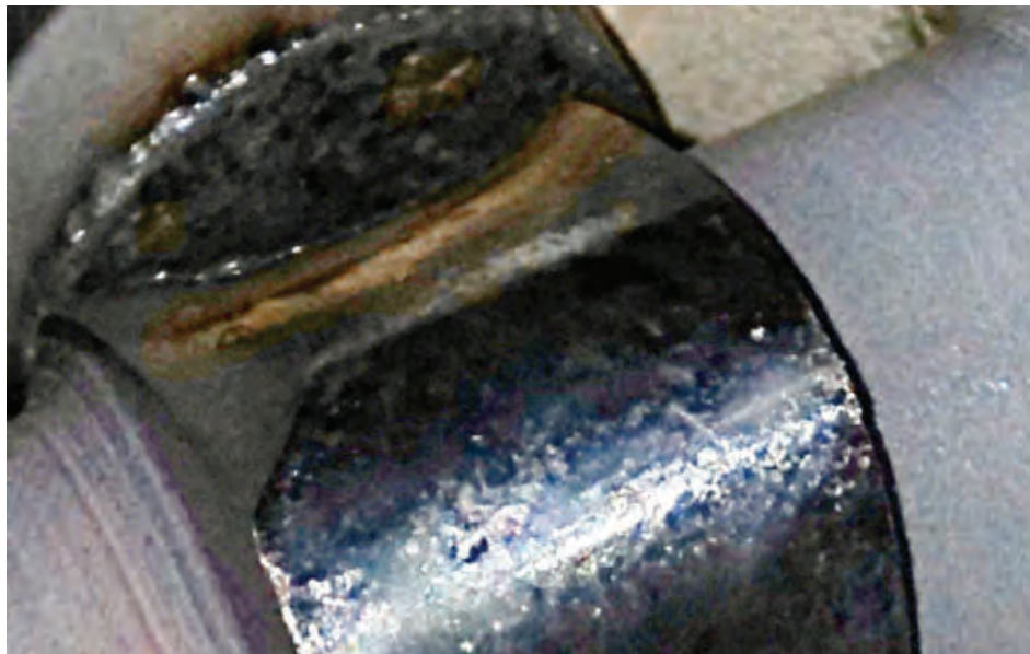
Figure 5—A higher-resolution image of the cam lobe, taken with a better camera and with better lighting, shows the cam lobe to be in worse shape than it originally appeared.
