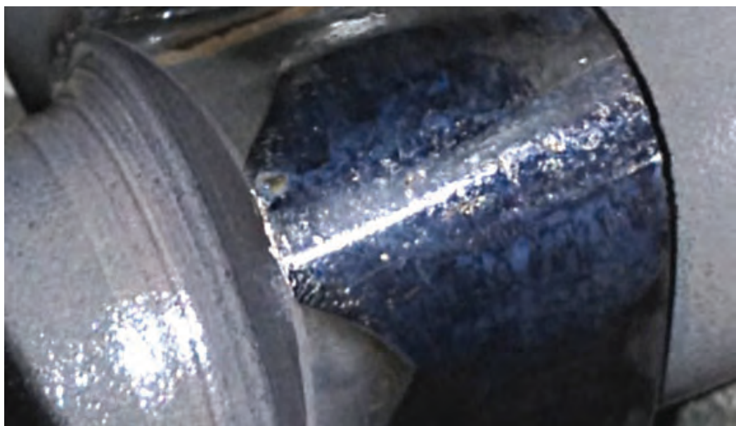
Figure 3—This close-up of the questionable cam lobe suggested that the distress is still minor and the engine could remain in service with 100-hour lifter inspections.
