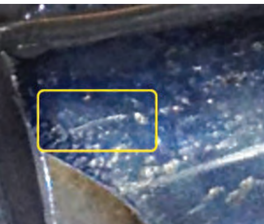
Figure 4—This close-up of the cam lobe at a slightly different angle reveals what might possibly be a surface crack—or perhaps just a piece of lint from a shop rag. The only way to know for sure is to probe it with a sharp pick.
