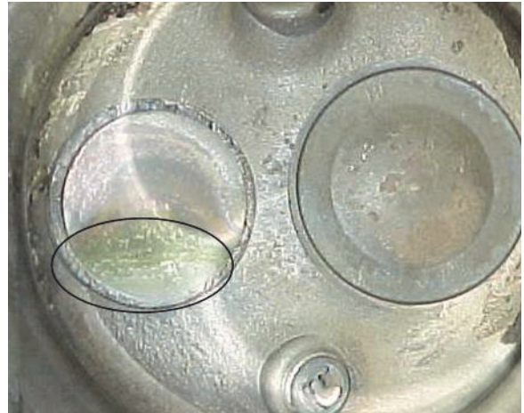
Figure 6-68. Burned Exhaust Valve
