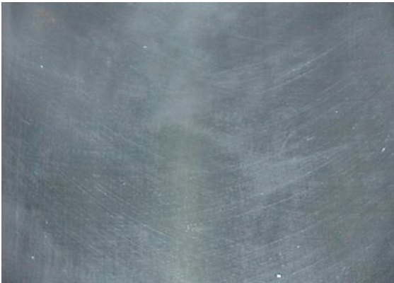
Figure 6-69. Phosphate-Coated Cylinder w/ Revised Hone Pattern
